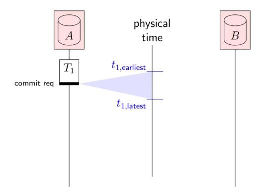
Spanner's TrueTime clock returns  $[t_{\text{earliest}}, t_{\text{latest}}]$ . True physical timestamp must lie within that range. On commit, wait for uncertainty  $\delta_i = t_{i,\text{latest}} - t_{i,\text{earliest}}$ .
